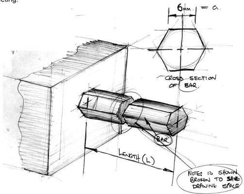
The figure above shows the bar projecting horizontally from a rigid mount in a vertical panel. The unsupported length of the bar L is 745mm. When viewed in cross-section, the hexagonal bar has equal faces of length a = 6 mm.
