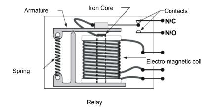
(ii) Explain how the parts interact to make the relay function.
