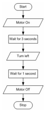
(a) Draw a fully dimensioned sketch of the path you would expect the robot buggy to take. Assume speed is constant.
