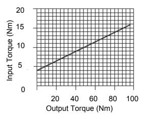
Use the graph to estimate the torque that the motor must deliver to hold the 600 N load off the ground.
