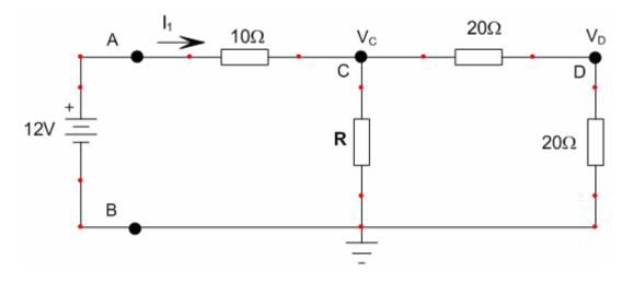
Note that node voltage  $V_C$  is the voltage drop from node C to the ground node; node voltage  $V_D$  is the voltage drop from node D to the ground node.
