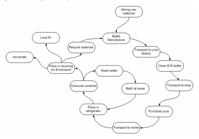
Each 'node' (labelled activities) in the diagram represents some action that is performed in the lifecycle of the plastic bottle. A 'pathway' shows the movement of the bottles between nodes. Each action may require energy inputs, and may generate energy outputs as well as waste and pollutants (solids, liquids and gases).
